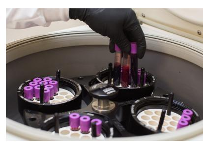
30 mechanical freezers at -80°C (~2 million samples), 17 liquid nitrogen tanks at -180°C (~ 1 million samples), a robotic freezer (pictured above) with 16 Ultra Low Temperature Units each at -80°C (> 4 million samples), and a smaller robotic freezer at -80°C for temporary storage and sorting of samples.
